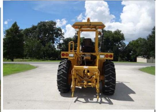
Built to withstand extreme applications, the frame accommodates multiple hitch configurations for high weight transfer, winches, and other equipment.
