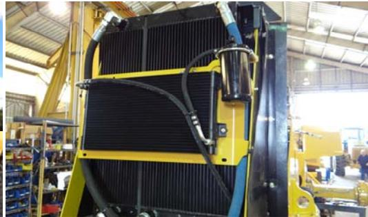
Engine and transmission coolers, with 8 fins per inch, spacing reduce buildup of debris. Hood rolls up for easy cleaning.
