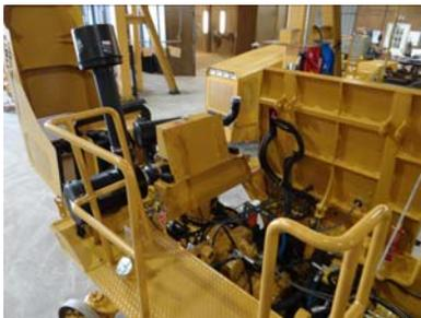
Tilting platform and hood provide unmatched access to engine, coolers, transmission, and under hood and cab components. Both work via hand pump even when systems are down.
