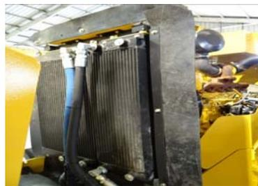
Engine and transmission coolers with 8 fins per inch spacing reduce buildup of debris. Hood rolls up for easy cleaning.
