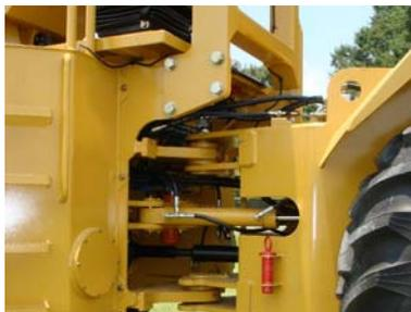
Extreme duty upper and lower articulation joint with radial spherical bearings, oversized hardened pins, and welded cylinders with bushings
