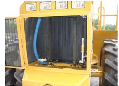
Engine and transmission coolers with 8 fins per inch spacing reduce buildup of debris. Coolers swing open for easy cleaning.
