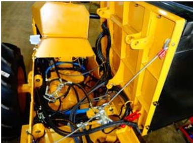
Tilting platform provides unmatched access to powertrain and hydraulic components
