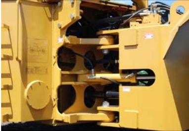
Extreme heavy duty upper and lower articulation joint with radial spherical bearings, oversized hardened pins, and welded cylinders with bushings
