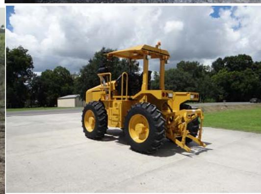
Tilting platform and hood provide unmatched access to engine, cooler and cab components. Both work via hand pump even when systems are down.
