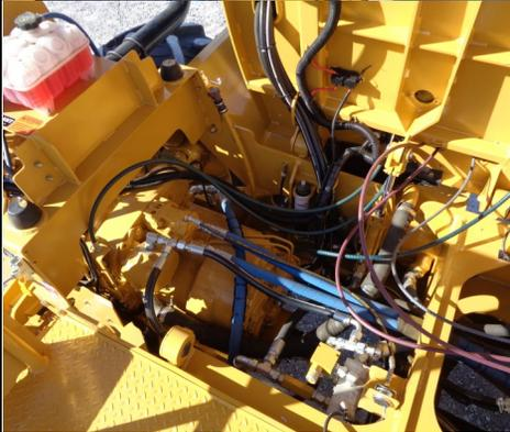
Tilting platform and hood provide unmatched access to engine, cooler, and cab components. Both work via hand pump even when systems are down.
