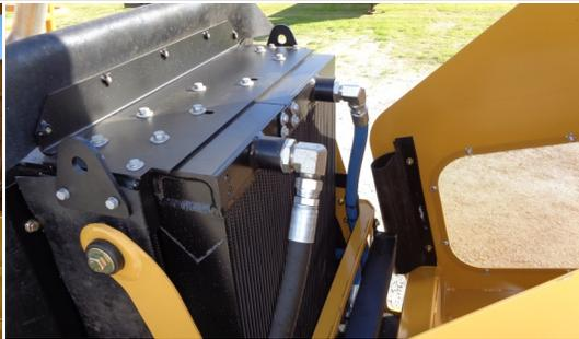
Engine and transmission coolers with 8 fins per inch spacing reduce buildup of debris. Hood rolls up for easy cleaning.
