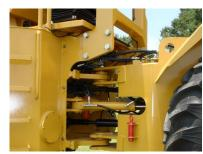
Extreme heavy duty upper and lower articulation joint with radial bearings, oversized spherical hardened pins, and welded cylinders with bushings
