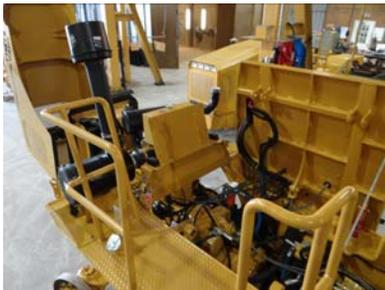
Tilting platform and hood provide unmatched access to engine, coolers, transmission, and under hood and cab components. Both work via hand pump even when systems are broken
