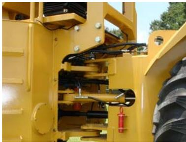
Extreme duty upper and lower articulation joint with radial spherical bearings, oversized hardened pins, and welded cylinders with bushings
