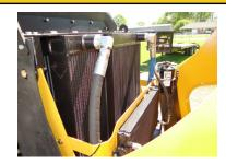
Engine and transmission coolers with 8 fins per inch spacing reduce buildup of debris. Hood rolls up for easy cleaning.
