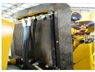
and transmission coolers with 8 fins per inch spacing reduce buildup of debris. Hood rolls up for easy cleaning.
