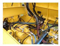
Tilting platform and hood provide unmatched access to engine, coolers, transmission, and under hood and cab components. Both work via hand pump even when systems are broken.
