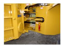
Extreme heavy duty upper and lower articulation joint with radial spherical bearings, oversized hardened pins, and welded cylinders with bushings.
