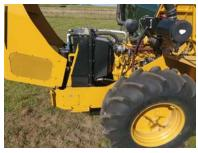
Engine and transmission coolers with 8 fins per inch spacing reduce buildup of debris. Hood rolls up for easy cleaning
