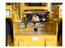
Rear frame accommodates multiple hitch configurations for high weight transfer, winches, and other equipment
