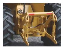
Optional drawbars and 3-point hitches are built to withstand extreme applications
