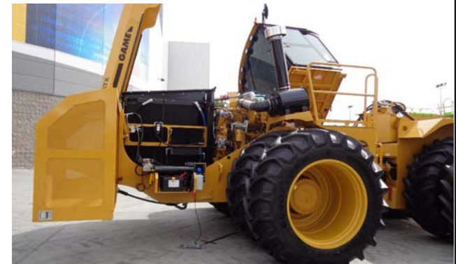
Forward tilting hood provides unmatched access to engine coolers and other components
