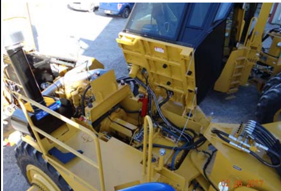
Tilting cab provides unmatched access to powertrain and hydraulic components
