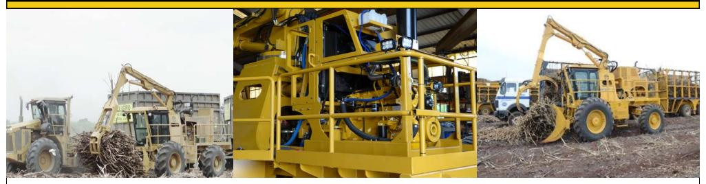
Large 1 Ton grab capacity increases efficiency.
