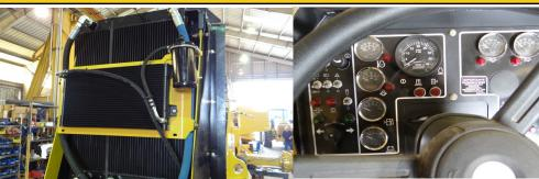
Engine and transmission coolers with 8 fins per inch spacing reduce buildup of debris. Hood rolls up for easy cleaning.
