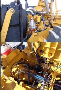
Tilting platform and hood provide unmatched access to engine, cooler, and cab components. Both work via hand pump even when systems are down.
