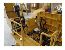
Tiltina platform and hood provide unmatched access to engine, coolers, transmission, and under hood and cab components. Both work via hand pump even when systems are broken
